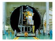
13m Ø Space Chamber (General Environment Test Building) This chamber is for checking the environment resistance of satellites in a space vacuum and thermal environment.
