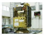
Large Scale Vibration Test Facility (General Environment Test Building) This facility is for conducting vibration tests on each satellite and rocket system or on parts of the system.
